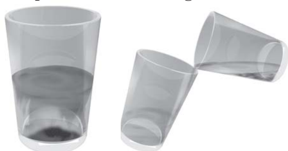
Fig. 5.8 Separating two components of a mixture by sedimentation and decantation
