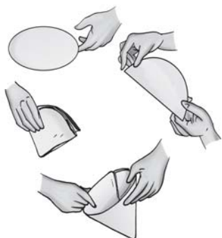
Fig. 5.9 Folding a filter paper to make a cone
