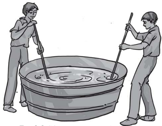
Fig. 3.8 (b) Scouring in tanks
