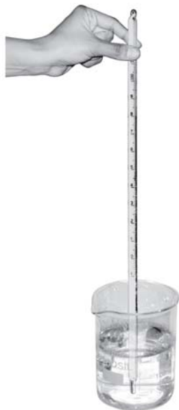
Fig. 4.5 Measuring temperature of water with an laboratory thermometer
