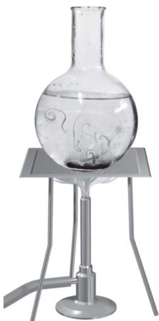
Fig. 4.9 Convection of heat in water
