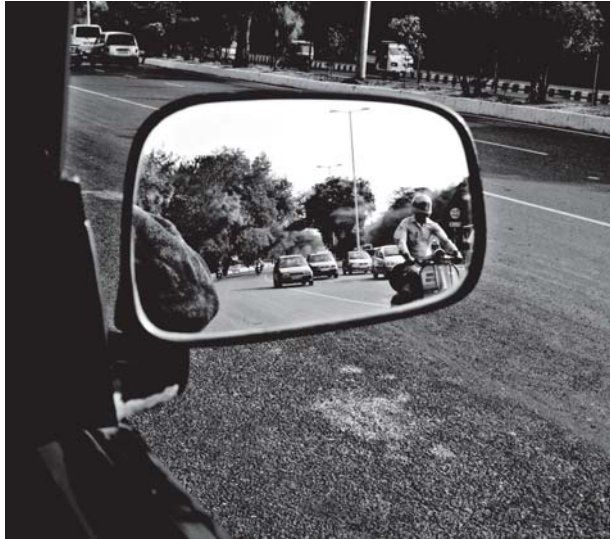
Fig. 15.20 Convex mirror as side view mirror
